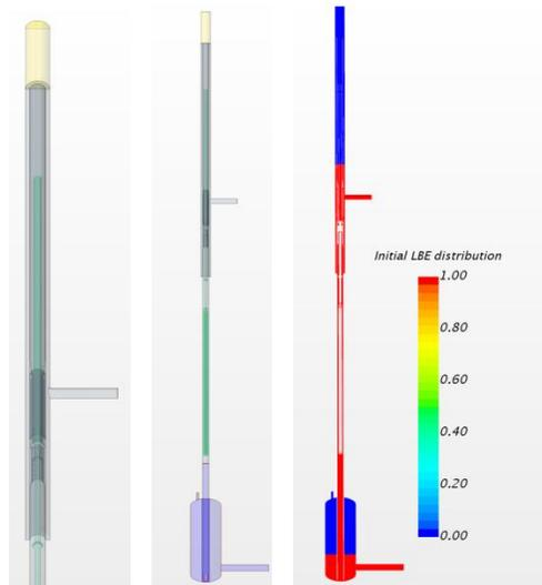
Fig. 3 Upper connected geometrical parts (left); overview of the complete computational geometry (center) and the initial distribution of the VOF phases (right)
