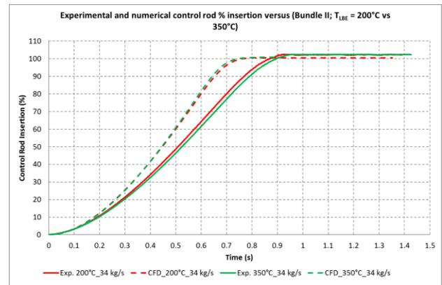
Fig. 9 Control rod insertion results at 200°C and 350°C: experimental versus numerical (Bundle II: 34 kg/s)
