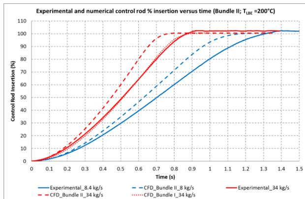
Fig. 8 Control rod insertion results at 200°C: experimental versus numerical (Bundle II: 8 kg/s and 34 kg/s)
