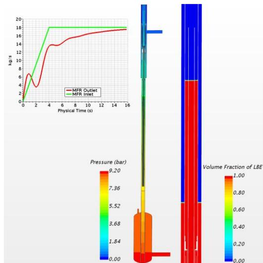
Fig. 4 Top left: history of the channels LBE filling with prescribed MFR= 36 kg/s (18 kg/s is shown due to the half domain); bottom left: free surface level in the buffer tank; center: partial filling of the guide tube; right: final LBE equilibrium level in the guide tube
