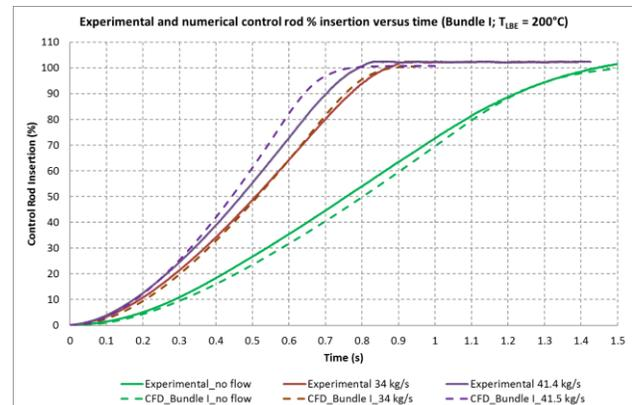
Fig. 7 Control Rod insertion results: experimental versus numerical (Bundle I) at 200°C
