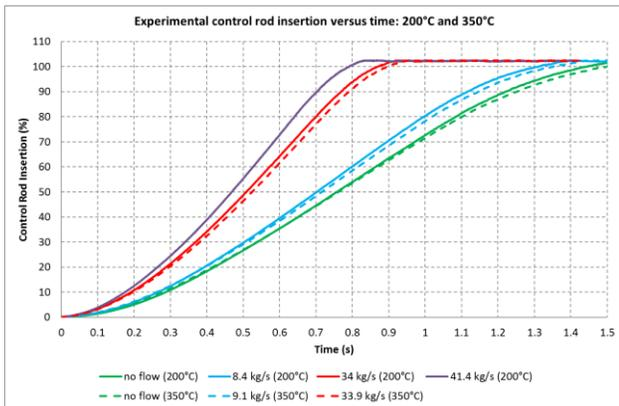
Fig. 5. Experimental CR insertion depth versus time – at LBE temperatures of 200°C and 350°C
