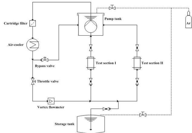
Fig. 1. Schematic of the COMPLOT loop
