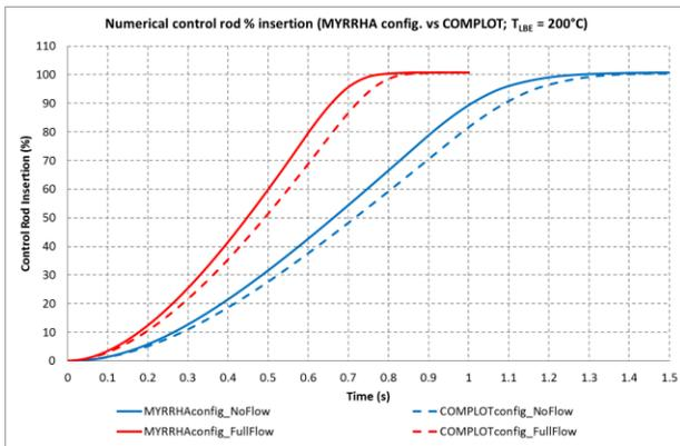
Fig. 10 Numerical MYRRHA configuration vs. numerical COMPLIT set-up. Rod displacement curves in two-way coupling motion (no flow and 37 kg/s)
