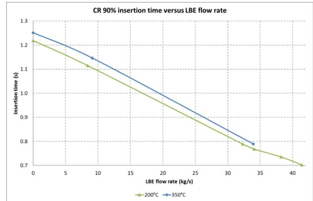
Fig. 6. Experimental CR insertion time for varying LBE flow rates, at LBE temperatures of 200°C and 350°C
